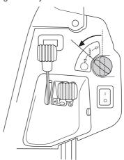
3 When the Rider is at a standstill, press down the parking brake and push in the locking button.
